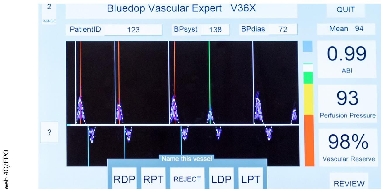
**Fig 2.** The output monitor device displays real-time results for each limb while scanning.
