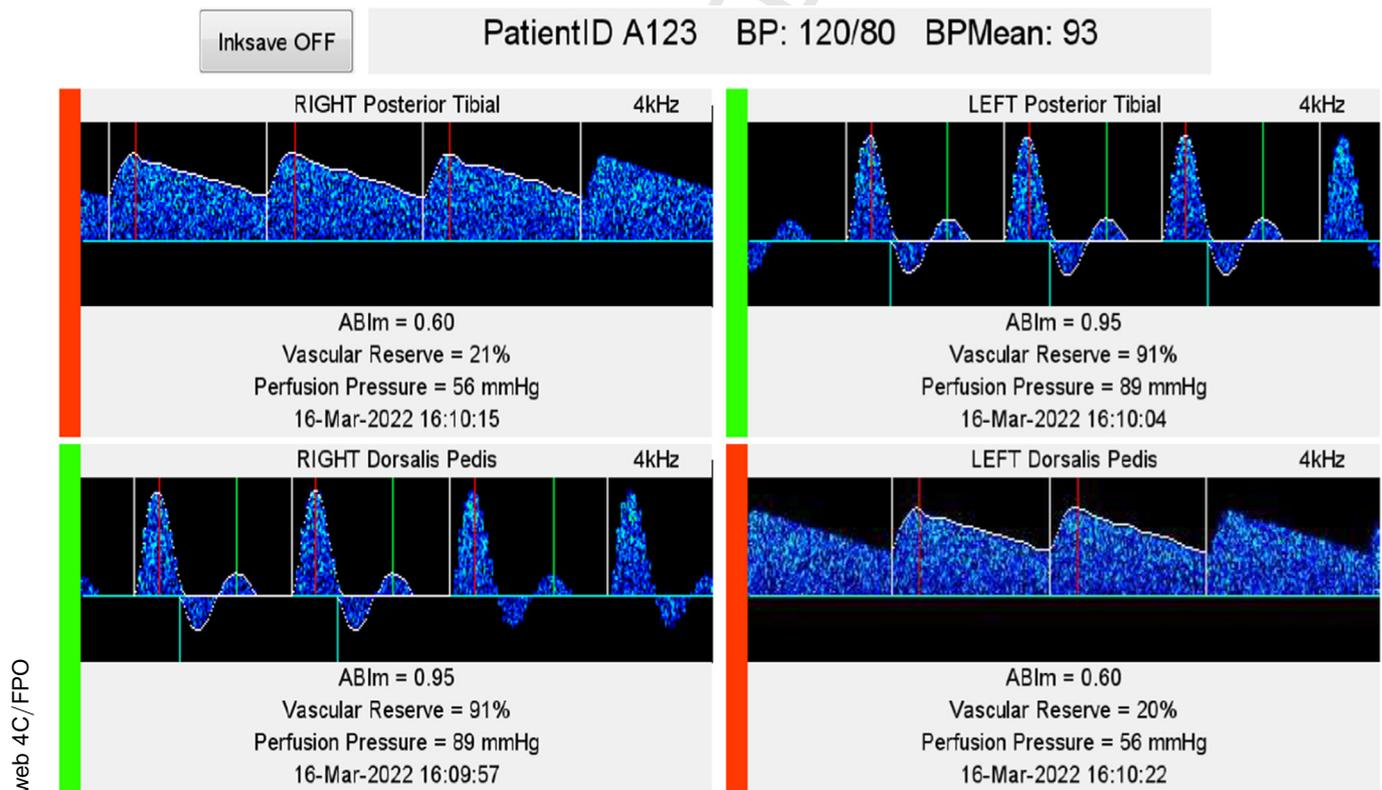
**Fig 3.** The output monitor is able to calculate full results with quantitative values such as the mean ankle-brachial index (ABIm), vascular reserve, and perfusion pressure, as well as the color-coded bars to indicate presence or absence of disease.
