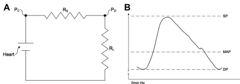
**Fig 4. (A)** Blood flow through vasculature is analogous to a closed electrical circuit. **(B)** Based on the same physics principles, BlueDop is able to measure the resistance and amplitude and calculate values like mean ankle-brachial index (ABI) through the validated pressure from flow algorithm.
